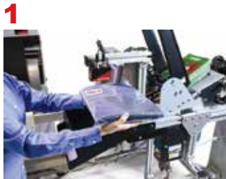
Product identifier is scanned.
