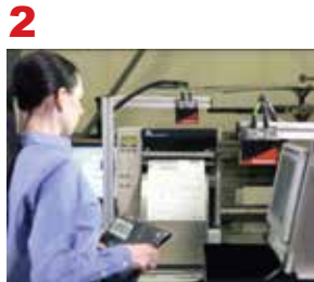
Packslip prints and drops into mailer automatically.
